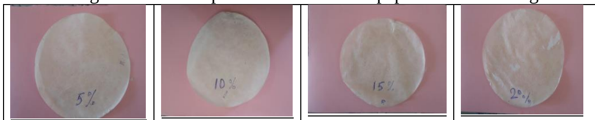
Figure no: 8. Impurities seen on filter papers after centrifuge.
