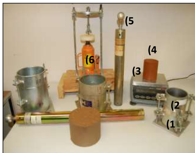
Fig. 1: the standard proctor apparatus
