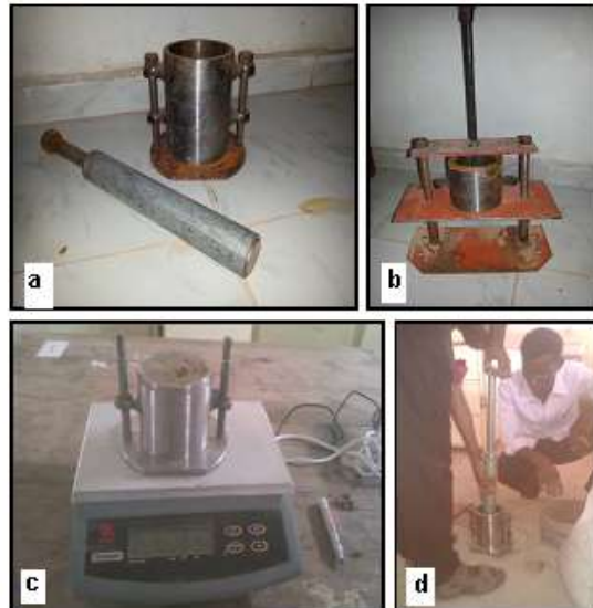
Fig. 4: the locally manufactured proctor apparatus
