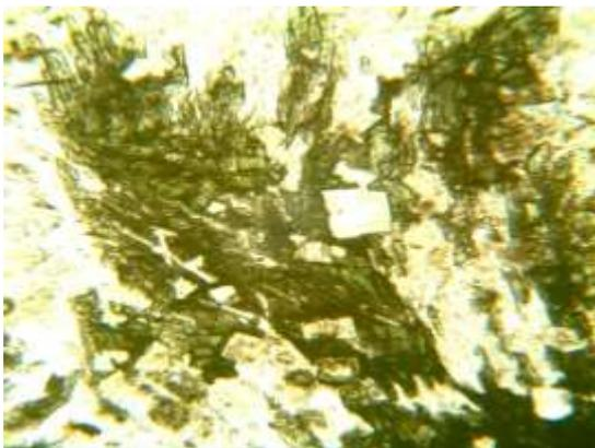
Plate (1a): Granitic gneiss-polarizer out. shows cracks-in quartz grains-polarizer in.
